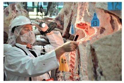
The Emroth Technologies Pty Ltd Chiller Assessment / Grading Torch has been developed to meet the harsh working environment of chillers. The use of powder coated aluminum torch body and battery case makes this a strong reliable work unit. The torch is controlled by electronic voltage sensing circuitry that automatically makes the torch flash when the battery starts to get low. The torch was developed with assistance from AUS-MEAT to ensure suitability for Chiller Assessment.
